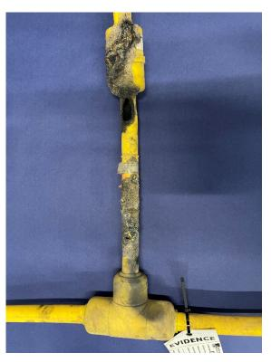
49. A photo of the melted gas supply line in the ground among the other partially uncovered parallel lines is as follows:
